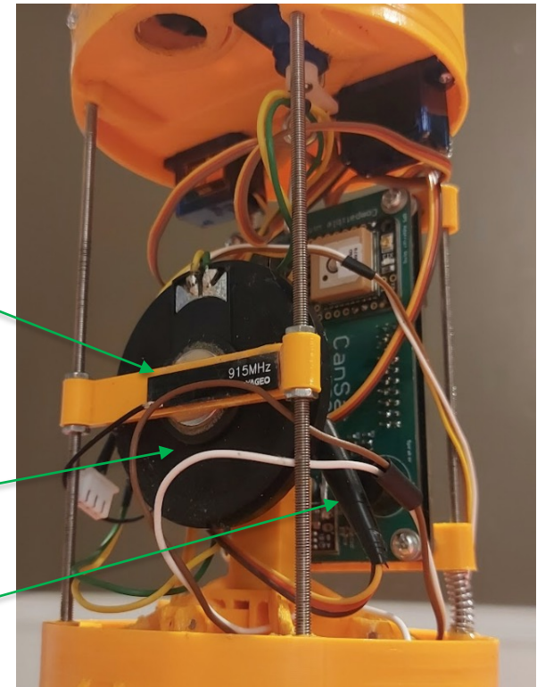
Rear of the electronics board with the antenna and buzzer visible
