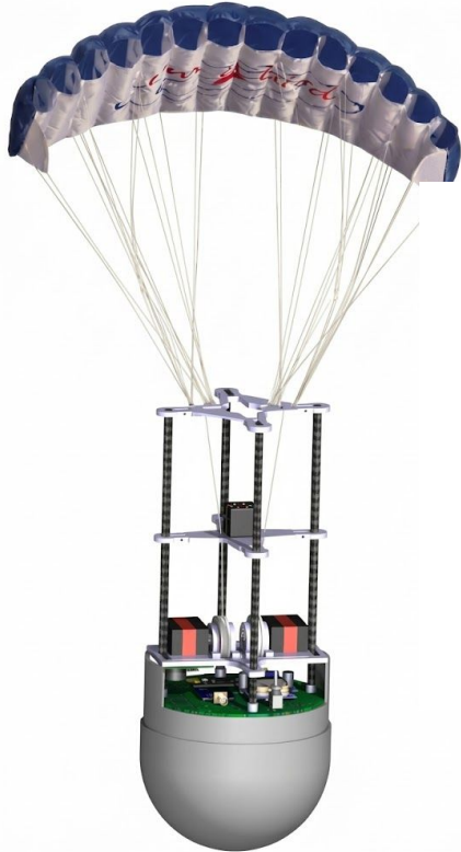
Payload and nose cone are held together by a fishing line
