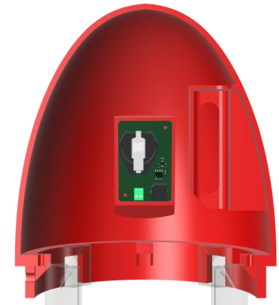
Placement of Beacon
