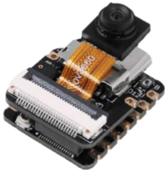
Sensor: OV5640 (1/4") CMOS 60° FOV
